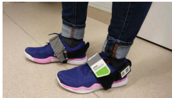
Figure 1. The RehaWatch® system with the sensors on the lateral side of the shoes.
