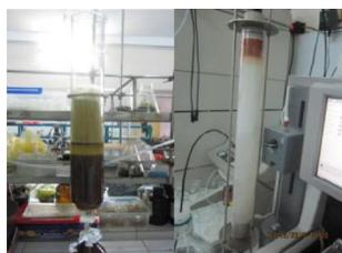
b) Column chromatography at atmospheric and high pressure
