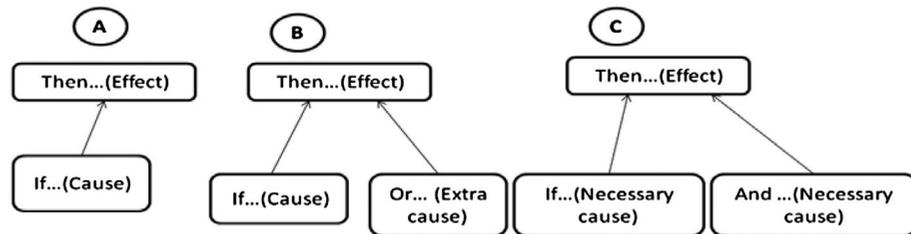
cause occurs, then the effect manifests itself. Lastly, the arrangement of letter C illustrates a sufficiency or insufficiency of cause, being understood: IF the cause occurs and the necessary cause, then the effect will occur.
