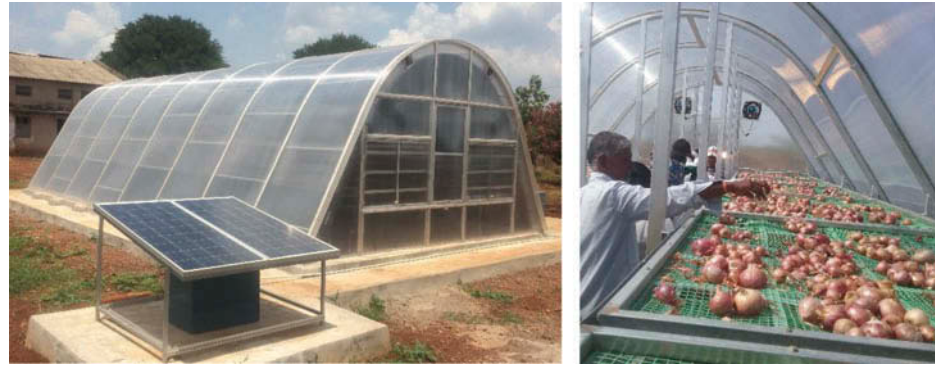
Figure 2. Greenhouse solar dryer in farmers' field in Vijayapura district (both outside and inside views—with onion crop).
