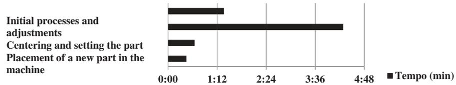
**Table 3. Comparison between the first and second footages of the setup process**
