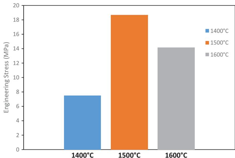
**Figure 7. Effects of sintering temperature on the absorbed energy of the ceramic samples.**
