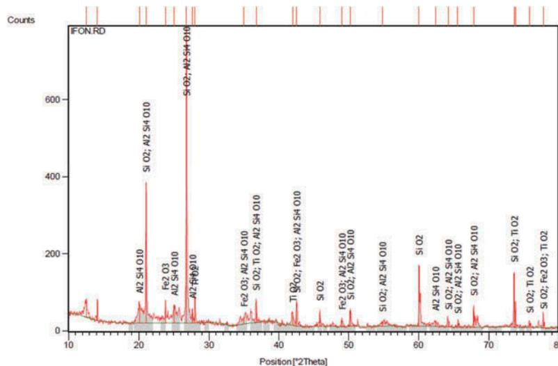
**Figure 2. Phases in samples D sintered at various temperatures.**
