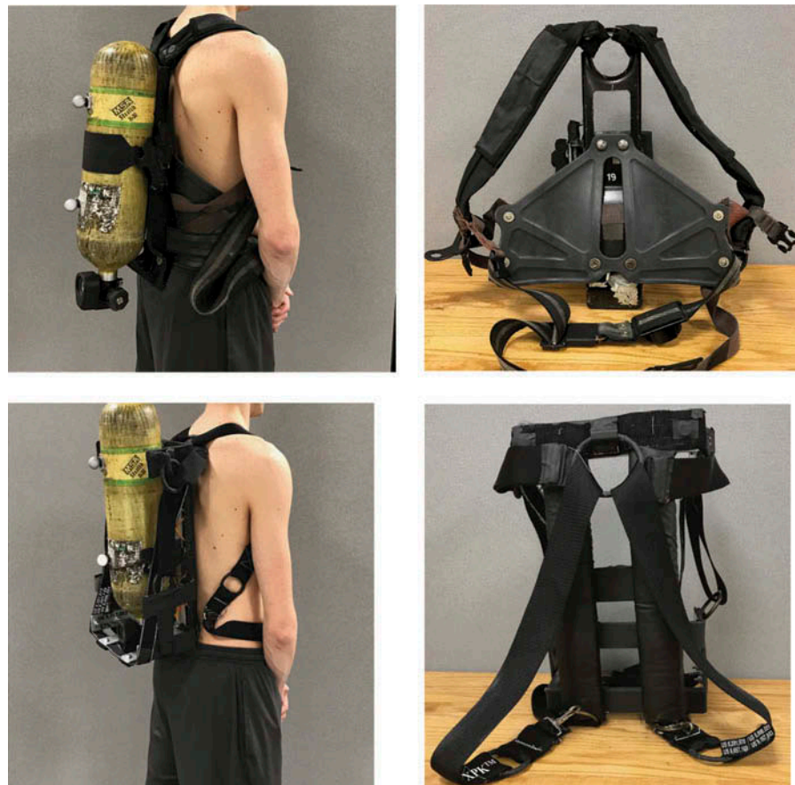
Figure 1. 1a (top: left and right). Traditional harness with padded shoulder straps and plastic frame attaching to tank clamp, and 1b (bottom: left and right). xPk® harness with aluminum frame with shoulder straps and padded back supports.
