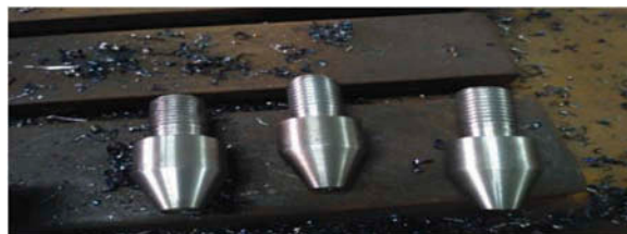
Figure 2. Carbide-coated nozzle in three different sizes.
