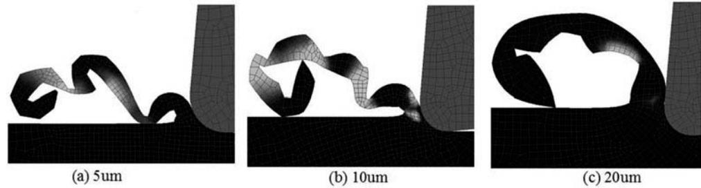
**Figure 9. Effective stress distributions in three different tool-tip radius (Unit: MPa).**
