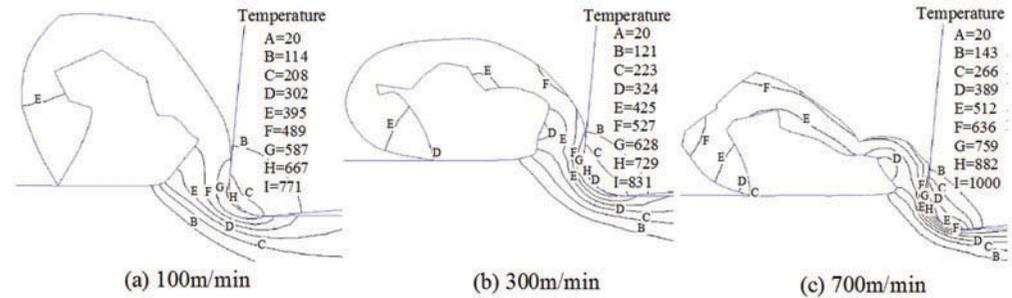
the cutting speed. Indicating that the maximum workpiece temperature increased from 632°C to 948°C, the maximum temperature of the tool increased from 228°C to 347°C, cutting speed from 100 m/min to 700 m/min. With the increase of cutting speed, the high temperature areas are concentrated on the chip-tool interface.
