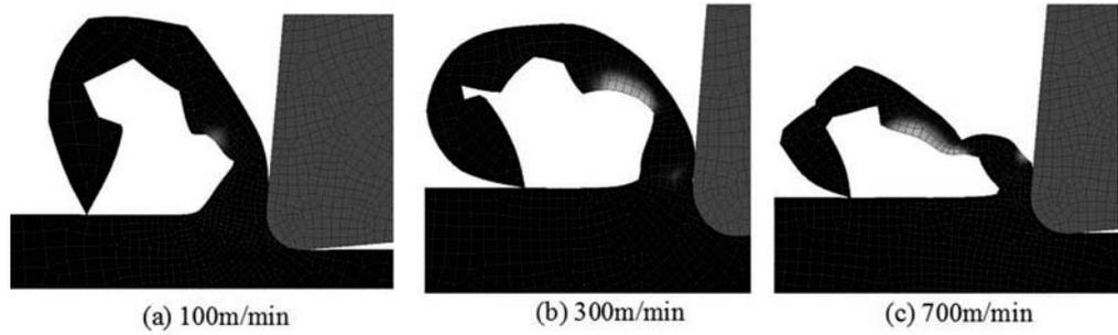
**Figure 3. Effective stress distributions in three different cutting speeds (Unit: MPa).**
