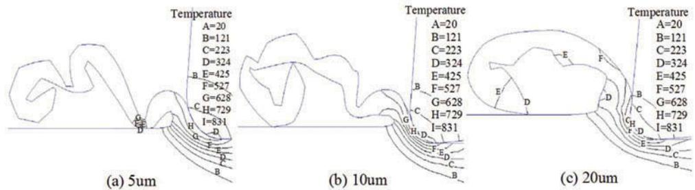
**Figure 4. Cutting temperature distributions in three different cutting speeds (Unit:°C).**
