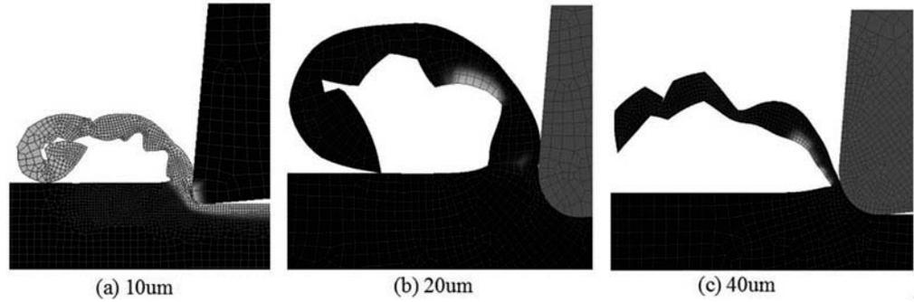
**Figure 6. Effective stress distributions in three different depths of cut (Unit: MPa).**
