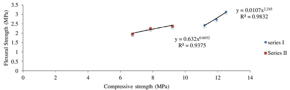
For the two series with GBS content, the best-fit relationships were found to be power correlations with  $R^2$  values ranging from 0.976–0.985. Figure 6 also shows that the best-fit correlation between the flexural and compressive strengths for the mixes with GGBS were found to be power relationships with  $R^2$  values ranging from 0.937–0.983.
