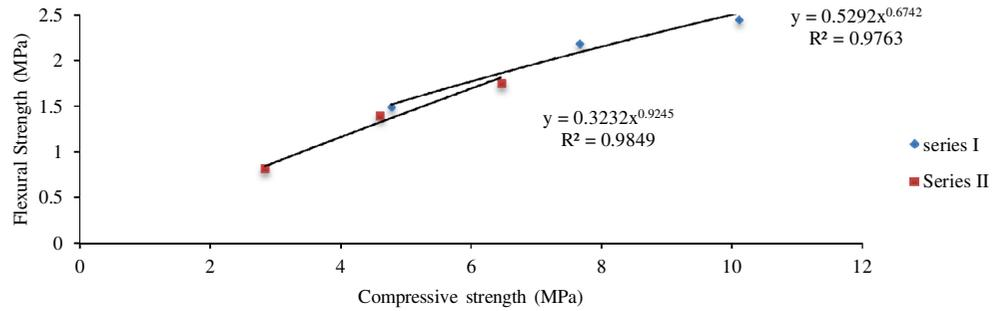
**Figure 6. Flexural strength at the age of 28 days as a function of its corresponding compressive strength for GGBS mixes in the two series.**
