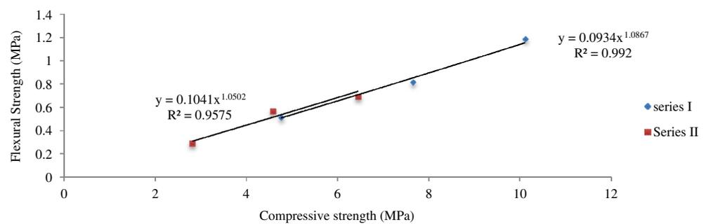
**Figure 10. Splitting tensile strength at the age of 28 days as a function of corresponding compressive strength for GGBS mixes in the two series.**
