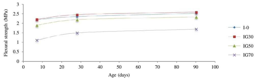
**Figure 4. Flexural strength as a function of age for GBS foam concrete mixes in Series II.**
