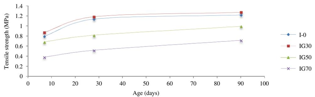
**Figure 8. Splitting tensile strength of GBS foam concrete for Series II as a function of age.**
