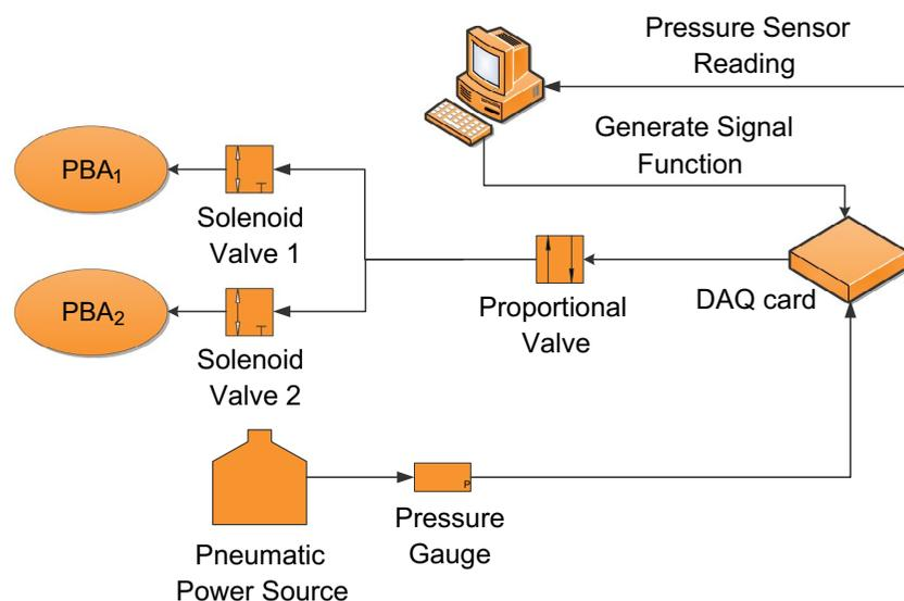
Figure 6. Closed loop control for the input pressure of the soft gripper.
