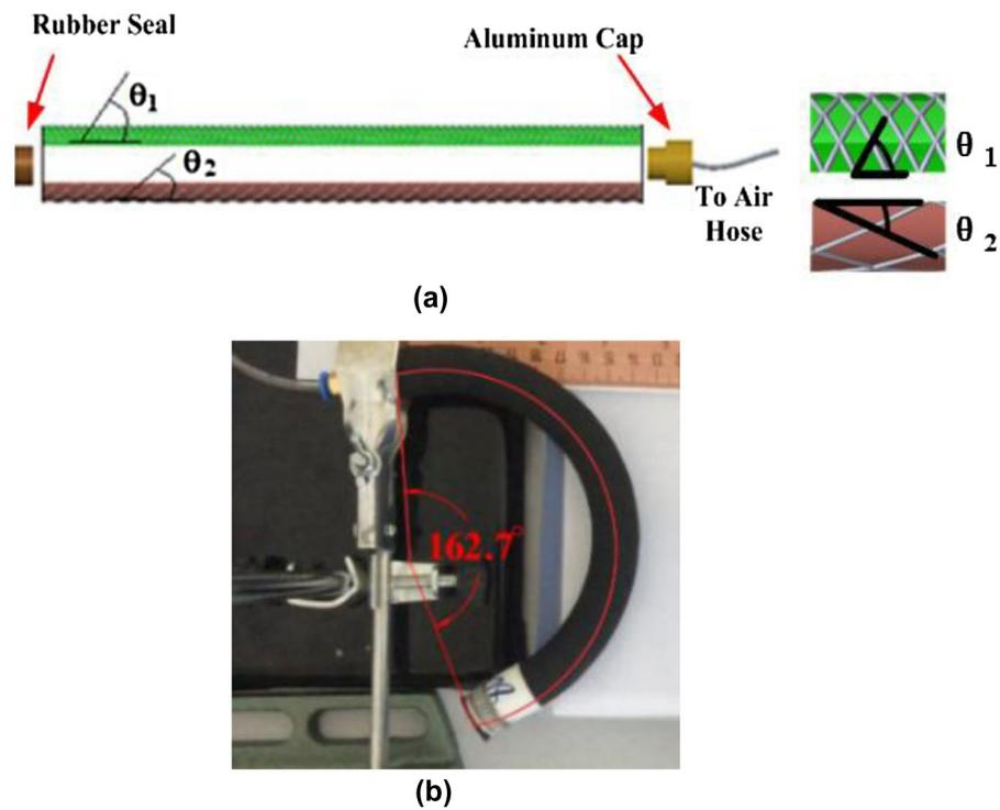
(referred to as extensible tubes); in contrast fiber reinforced rubber tubes with  $\theta$  less than  $54.7^\circ$  contract length-wise on pressurization (contractile tubes). Using this principle bending actuators can be produced by slitting the tubes in half lengthwise and bonding half a contractile rubber tube to half an extensible rubber tube.
