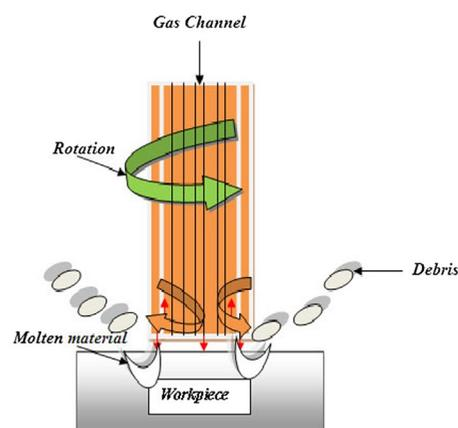
Most likely advantages of DEDM process are negligible tool wear, low residual stresses and better precision. For machine makers and machine user's practical application of the DEDM process strive many advantages like simplicity in machine building, it does not require advanced and spacious dielectric circulation and cooling mechanism, thus contributes to reduction in manufacturing cost.
