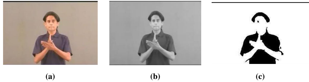
Figure 4. Sign gesture recognition for meat : (a) input frame, (b) noise removed, output, (c) segmented output.
