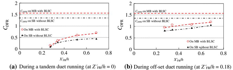
**Figure 7. Distribution of drag ratio  $\eta$  behind a preceding runner during duet running compared to solo running (at  $Re = 1.0 \times 10^5$ ).**
