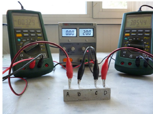
Figure 2. Four poles resistivity testing, after Konsta-Gdoutos and Aza (2014).
