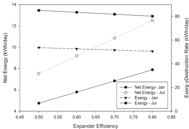
Reducing the turbine efficiency reduces the net energy produced and slightly raises the total exergy produced. The percent decrease of net energy produced did not vary from January to July. The percent decrease from reducing the efficiency from 80 to 70% was 13% for both January and July, while the percent increase of the total exergy destroyed was 2%.
