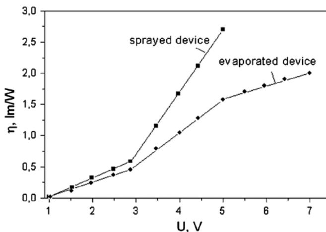
The resulting luminance efficiency for both devices is shown in Figure 6. As can be seen for the device with sprayed layer the throughput can be increased average by 30%. This is ascribed to the optimized spray deposition conditions, leading to smooth and uniform EL films and resulting in lower contact resistance, higher conductivity, and smaller voltage drop at the electrode interfaces in comparison to OLED with thermally evaporated EL films.
