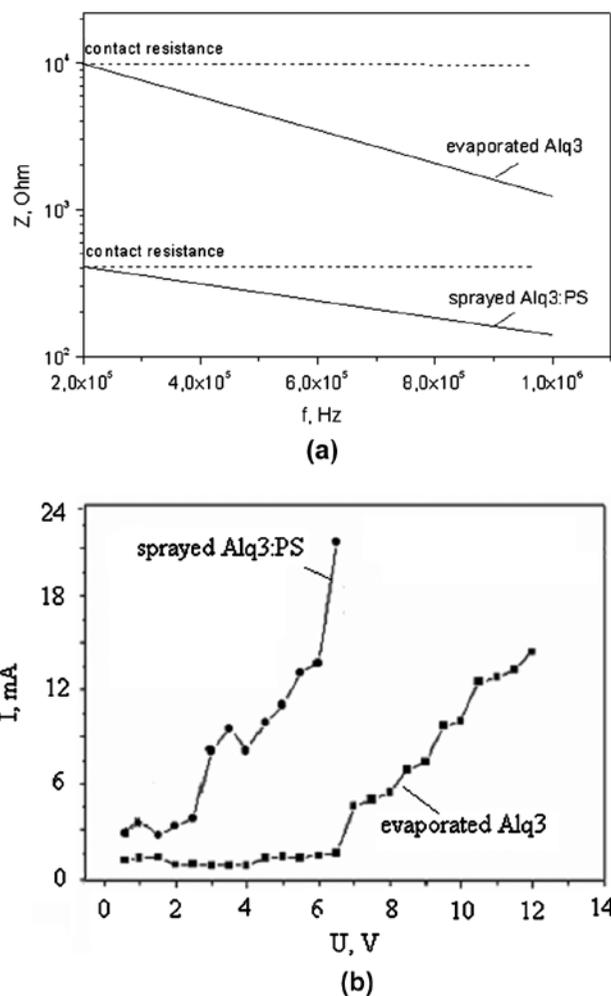
shows the capacitive behavior of the devices. It is related to the junction capacitance, which affects mainly on the delay times at on-off switching conditions and vice versa. However, the process of interfacial capacitance recharging is out of the scope of this work and it is not given.
