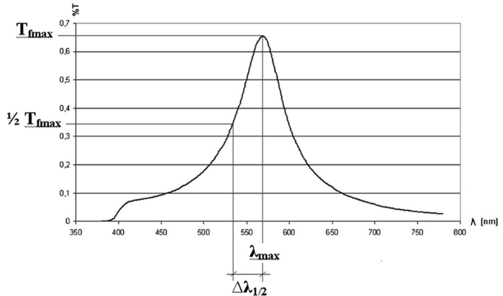
Figure 3. Transmission characteristics  $T(\lambda)$  of a metallic reflective filter (protection level 4–5).
