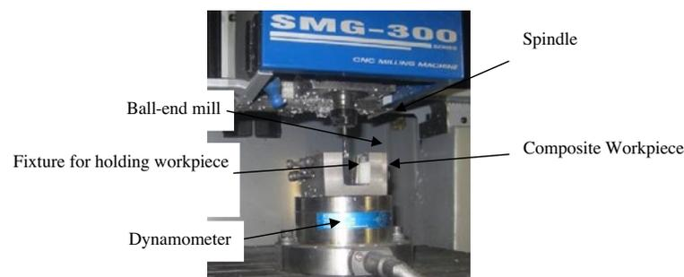
Figure 3. Photograph of milled workpiece.
