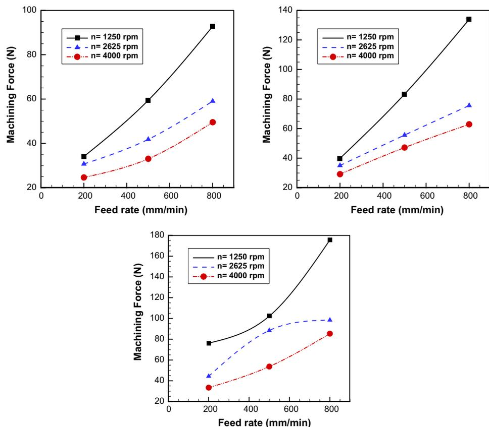
cutting speed on temperature rise at the cutting edge in GFRP cutting were found (Sakuma & Seto, 1981). So by increasing the temperature, due to increase in cutting speed, the cutting force is decreased.
