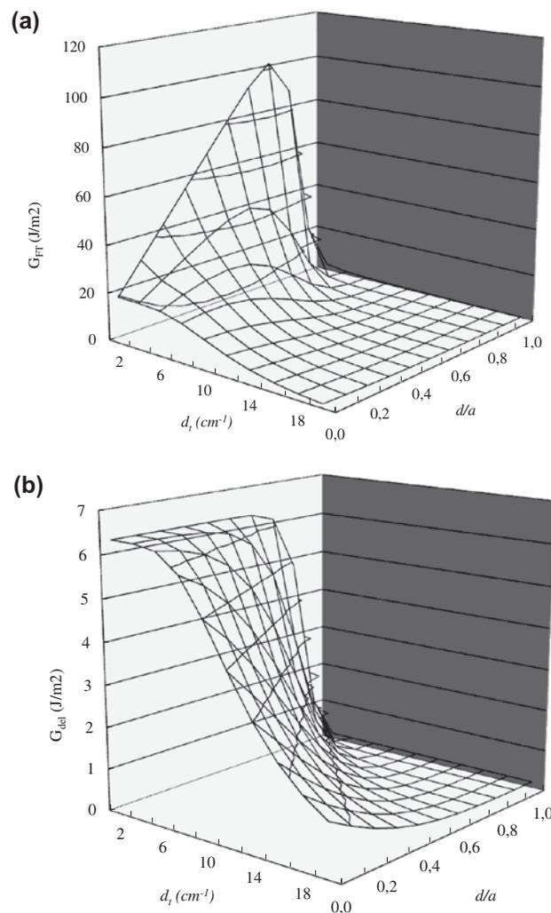
**Figure 3. Strain energy release rates  $G_{FT}$  and  $G_{del}$  vs. constraining parameter  $\lambda$  (a) graphite/epoxy system and (b) glass/epoxy system.**
