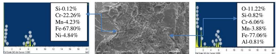
(C) SEM image at 105MPa axial pressure
