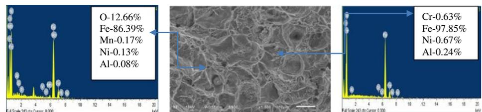
(E) SEM image at 135MPa axial pressure
