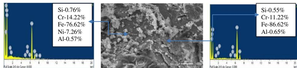
(A) SEM image at 75MPa axial pressure
