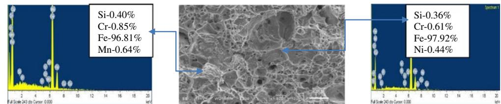
(D) SEM image at 120MPa axial pressure
