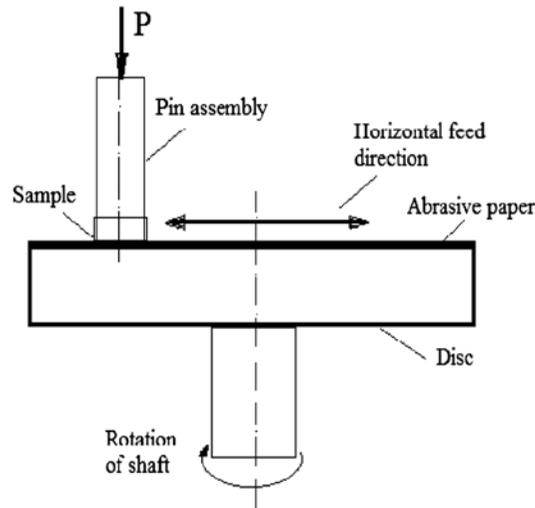
$$K_s = \frac{\Delta M}{\rho L F_n} \left( \frac{\text{mm}^3}{\text{Nm}} \right) \quad (2)$$
