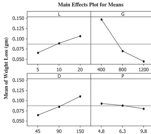
**Figure 4. Main effects plot for average the volume loss of polymer composites.**
