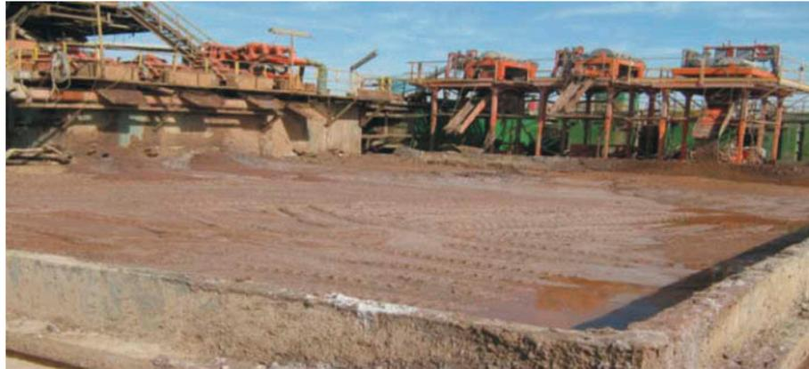
130 cubic meters can produce a suitable response for a large volume of mud in a critical condition. Discharged particles in this site are ultimately managed by stabilizing chemicals such as cement and sodium silicate.
