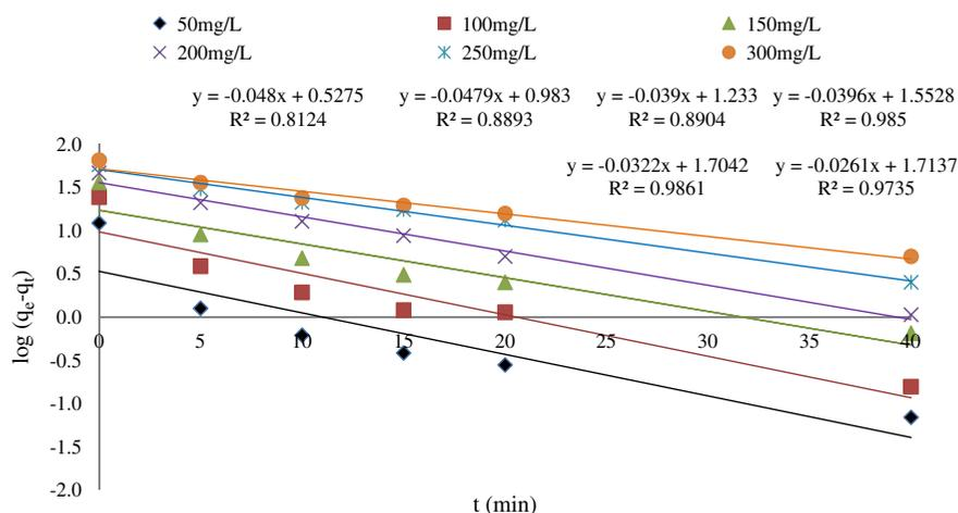
**Figure 12. Pseudo-second-order kinetic model for different initial MB dye concentrations onto sawdust.**
