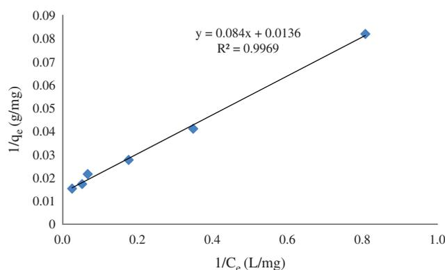
Figure 7. Freundlich isotherm plots for MB dye adsorption onto sawdust.
