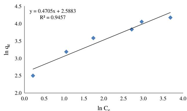
**Figure 8. Temkin isotherm plots for MB dye adsorption onto sawdust.**
